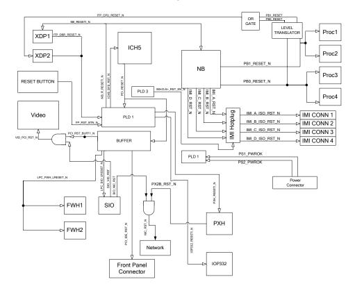
Figure 16. Reset Block Diagram
